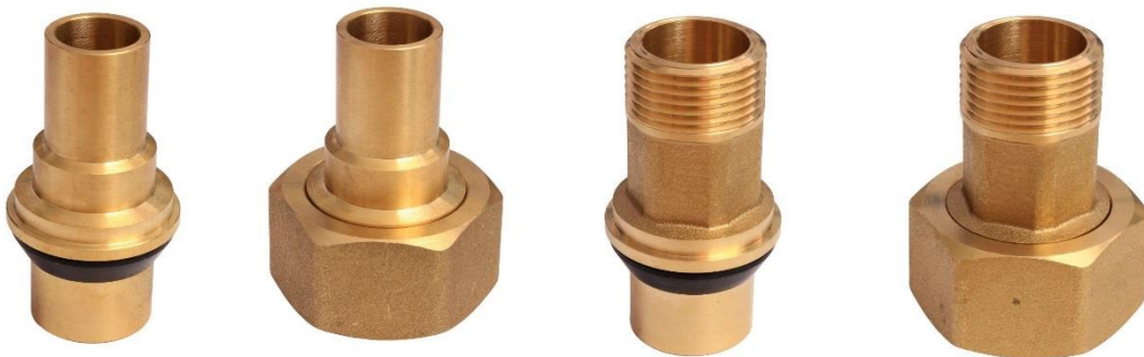
Picture above show an example of two types of ECV adaptor to allow the meter install to take place – both with a BS746 outlet thread and 22mm capillary – the ECV does not require changing if it is fully functional and not leaking.
