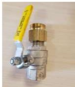
3/4" female BSP Taper x 3/4" male BSP Taper Valve with 3/4" female BSP Taper x 3/4" BS746 adaptor fitted. (Same adaptor can be used for angled valves with 3/4" male BSP outlet thread).
